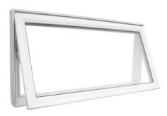
Sash is hinged on the top enabling the window to be open in many weather conditions, even when raining. The top hinge design gives protected air flow while providing the same performance as the casement style. Same profile and design as the Casement.
