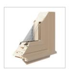
Insert Installation: The Trinity® Series platform is based on a 31/4" frame profile that makes it the right fit for replacing windows within an existing window frame while leaving the home's interior and exterior original finishes.
